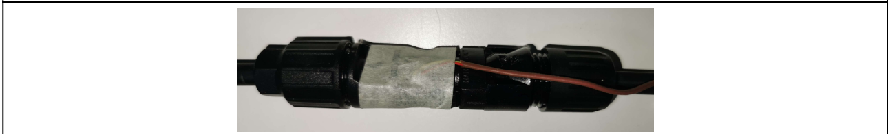
Couple 1 Photo during temperature test – Thermocouples applied on case of connector The samples provided are all the same n.3 samples (male-female combination) identified 1A - 2A - 3A during the tests. Cable length 1400mm - 6mm 2
