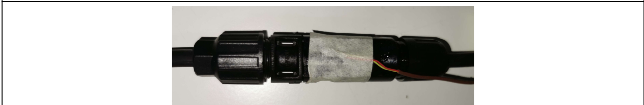
Couple 2 Photo during temperature test – Thermocouples applied on case of connector The samples provided are all the same n.3 samples (male-female combination) identified 1A - 2A - 3A during the tests. Cable length 1400mm - 6mm 2
